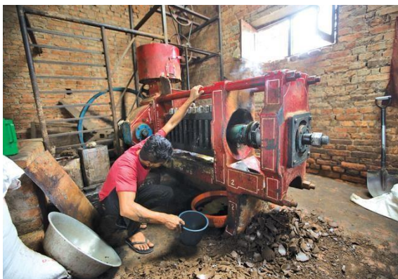
Figure 2.16 Oil cake collected by 2 nd press by mechanical process
