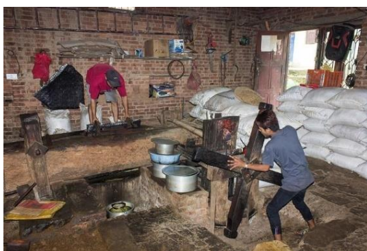
Figure 2.12 Workers putting pau in middle of stone and moving chakra to press pau at the same time
