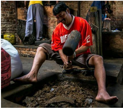
Figure 2.14 Hammering oil cake for 2 nd press
