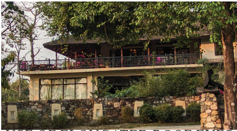
USE OF ELONGATED ROOF EVES TO CONTROL SUN RAYS AND INTERIOR TEMPERATURE
