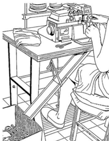
Figure 2.62: Litterbox attached to workstation
