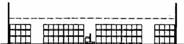
Figure 2.30: Fork-lift in pallet racking
