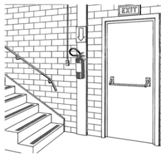
Figure 2.54: Fire extinguisher near the exit door (Source: International Labour Organization, 1998)
